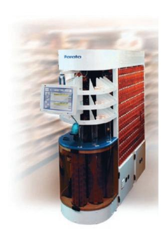
The Parata RDS (Robotic Dispensing System) is a next-generation prescription processing technology that accurately automates more than half of a pharmacy's prescription load. The Parata RDS processes a prescription in just 20-25 seconds, including labeling, filling, capping and sorting by patient last name. With Parata patients benefit from shorter wait times and more time with the pharmacist to learn about their prescriptions, disease management or related issues.
